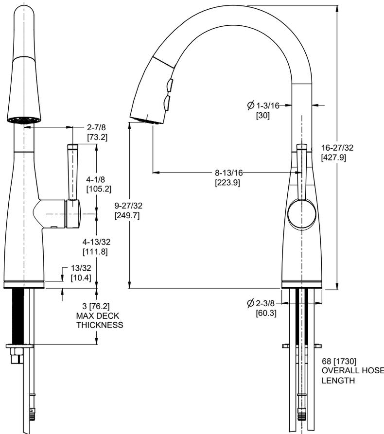
$\text{Ø}1\text{-}3/8$  Min to  $\text{Ø}1\text{-}1/2$  Max. Deck Hole Openings
